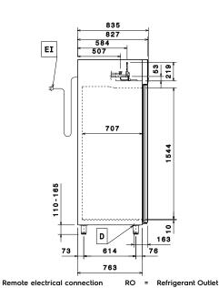
ED ΕI Electrical inlet (power) Refrigerant Inlet
